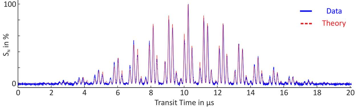
Figure S1: **Normalized scattering signal of a freely rotating nanorod.** Simulated signal as a function of time (red dashed line) in comparison to experimental data (blue solid line). The following parameters and initial values were assumed:  $E_0 = 4.15 \times 10^6$  V/m,  $v_x = 11.5$  m/s,  $z(0) = -89.85/k$ ,  $\dot{z}(0) = 0.74$  m/s,  $\phi(0) = 0.1$  rad,  $\dot{\phi}(0)/2\pi = 2.14$  MHz.
