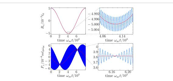
**Figure B1.** In the limit of high drive frequencies, the center of mass performs an approximately harmonic oscillation. The exact trajectory and momentum oscillations (dark blue solid line) are very well described by the macromotion dynamics (red solid line) if the momentum correction (54) is included (light blue dashed line).
