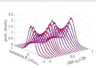
Figure 4. Equilibrated center-of-mass momentum  $P_z$  distribution as a function of time in the ring-shaped Paul trap for vanishing dipole moment. The full time-dependent stochastic dynamics (red) are determined by the AC voltage  $qU_{\rm ac}/m\omega_{\rm ac}^2\ell_0^2=0.0034$ , the environment temperature  $k_{\rm B}T/m\omega_{\rm ac}^2\ell_0^2=0.034$ , and the linear damping rate  $\Gamma/\omega_{\rm ac}=0.02$ . The analytic distribution (62) is shown in blue.
